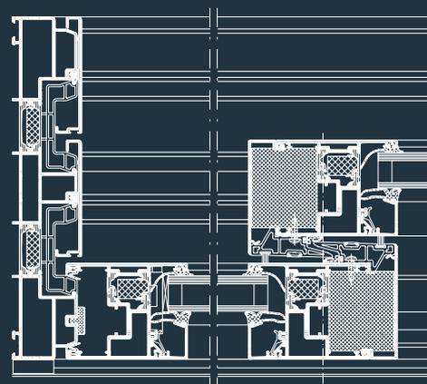
Schüco Hebe-Schiebesystem ASS 70.HI, M = 1:5
